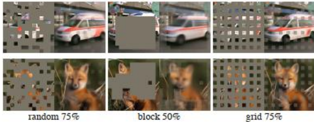
Figure 6. Mask sampling strategies determine the pretext task difficulty, influencing reconstruction quality and representations (Table 1f). Here each output is from an MAE trained with the specified masking strategy. Left: random sampling (our default). Middle: block-wise sampling [2] that removes large random blocks. Right: grid-wise sampling that keeps one of every four patches. Images are from the validation set.
