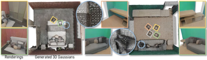
Fig. 1. L3DG learns a compressed latent space of 3D Gaussian representations and efficiently synthesizes novel scenes via diffusion in latent space. This approach makes L3DG scalable to room-size scenes, which are generated from pure noise leading to geometrically realistic scenes of 3D Gaussians that can be rendered in real-time. Above results are from our model trained on 3D-FRONT; we visualize the 3D Gaussian ellipsoids and show renderings.
